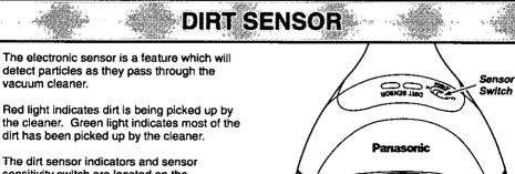
sensitivity switch are located on the topt of the switch cover. See the Dirt Sensor section under To Operate Cleaner section for operation.
